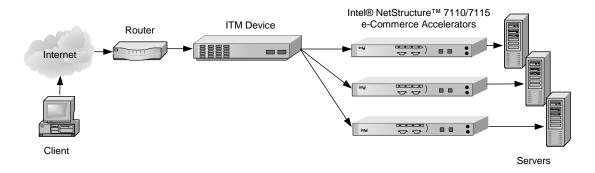
NOTE: The configuration in Figure 1-4 precludes layer 7 load balancing because secure traffic through the ITM device is encrypted.
